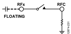
Figure 63. Series Capacitor Directly Connected to MEMS Switch
