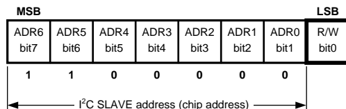
Figure 21. I 2 C Chip Address (see NOTE above)
