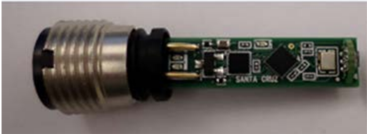
Figure 8. The MAXREFDES23# is a tiny IO-Link light sensor that integrates six sensors: ambient light (clear), red, green, blue, infrared, and temperature. All are on a tiny printed circuit board (PCB) that is 6.5mm x 25mm.
